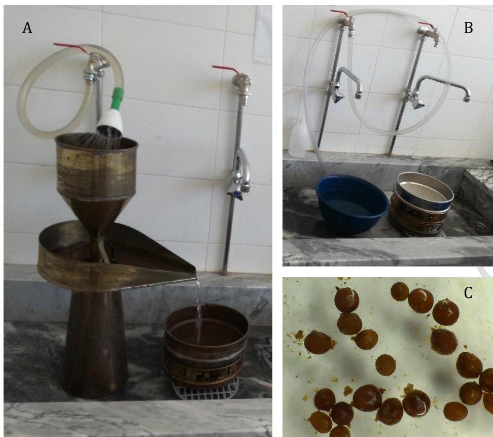
Figure 1. Extraction methods. A: Fenwick can; B: Cobb's decanting and sieving technique; C: cysts collected.
